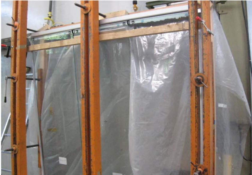
Fig. 1 Top rail drawn out from height compensation profile at 4000 Pa, height compensation profile deformed, right-hand pane broken when hitting the test rig, cover sections disengaged.
