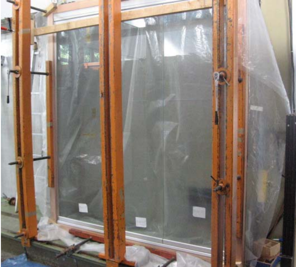
Fig. 11 Test setup for static wind load
