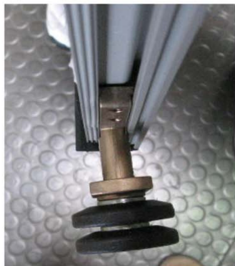
Fig. 3 Guide runners permanently deformed
