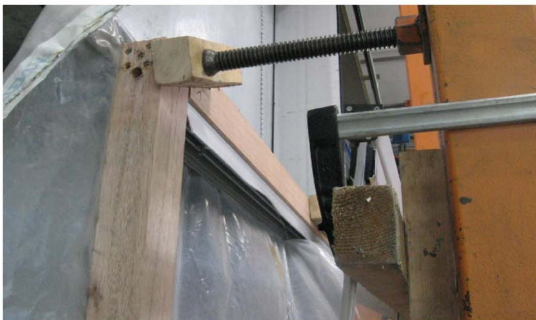
Fig. 1 Top rail drawn out from height compensation profile at 2300 Pa, height compensation profile deformed.
